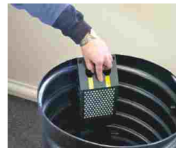
Remove the front plate by sliding upward
